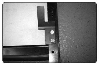
Loosely fix brackets to the back of the seat frame using nuts and bolts only.
