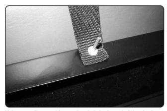
Using a small screwdriver make a hole in the end of the check strap and rivet the strap to the centre of the base frame.
