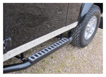
8. Test the step before you put it to use. Ensure all bolts are tight, and the tube lugs are correctly aligned. Although our steps are coated and galvanised to protect against rust, we recommend using Hammerite to coat the arms for additional longevity.
