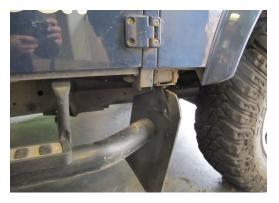
6. Check alignment of step; then tighten all nuts and bolts. The sills do not necessarily need to be removed.
