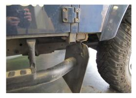
1. Offer the step into place on the outer edge of floor rails, the front hole is clear, the last rear hole in the rail needs the factory nut and bolt removing. The sills do not necessarily need to be removed.
