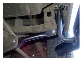
2. If your Defender has a fuel tank on the driver's side then the front fixing bolt should be pushed through from up behind the tank.
