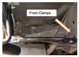
3. Fit the long front brace with clips underneath, and clamp to the edge of the tapered front chassis flange by the big rubber bush.
