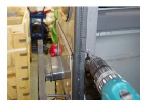
7. Fix the rear quarter panels in place with three long screws using the holes drilled in the previous step.
