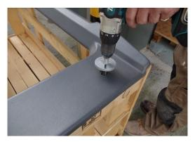
2. Offer each side trim up to your Defender and mark out the seat belt aperture points. Carefully drill out the points.
