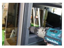
6. Set the first rear quarter panel in place and drill three small holes, as shown in the image above. Repeat this process on the other side of the vehicle.
