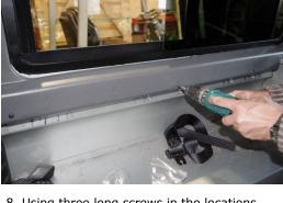
8. Using three long screws in the locations shown in the image above, fix each side panel in place. Take care not to over tighten these screws as the plastic could crack.
