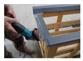
4. Offer all four trim panels to their respective surfaces. If the trim does not quite fit or is obstructed by anything on the interior of the vehicle, carefully file off any excess material with an angle grinder until the panel fits comfortably.
