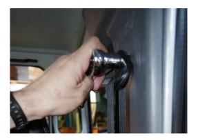
5. Set the first side panel in place and, once you are happy that it fits, reattach the seat belt bracket to hold it in place. Repeat this process on the other side of the vehicle. Slide the rubber seals in to finish off the edges of the trims. (To the right of the trim in the photo above.)
