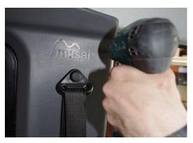
9. Secure the front edge of each side panel using two shorter screws—one in the top and one in the bottom.
