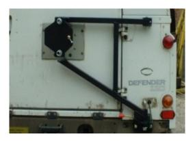
1. Place the wheel carrier in position with the bottom bracket on the rear cross member straddling the body lug.
