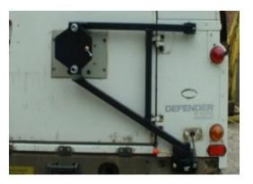
8. Place the wheel carrier in position and using the two M10 bolts, bolt the bottom bracket to the cross member using the backing plate between the cross member and the nuts.
