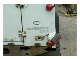
2. Make sure the top bracket is level and over the reinforced joint between the body tub and the hardtop or canvas tilt. Note, if the vehicle is fitted with a rectangular rear fog light, this may need to be raised to provide clearance.
