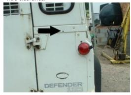
4. Remove the wheel carrier and measure the distance between centres of top bracket holes. It should be 40mm. Use this measurement to mark the position of the other hole in top bracket.
