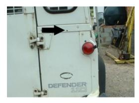
6. Enlarge the top holes using a 7mm drill bit to accept the 6mm bolts and use a 10.5mm drill on the cross member to accept the 10mm bolts, making sure you drill through both sides of cross member.
