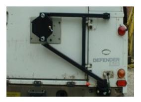
10. If required, two additional holes can be drilled through the backing plate using a 7mm drill and the bracket can be secured using the two M6 Posi-head bolts.
