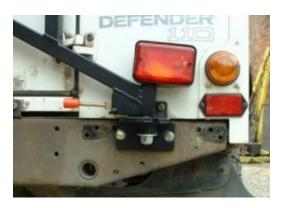
7. Remove any burrs and touch up any bare metal with paint.
