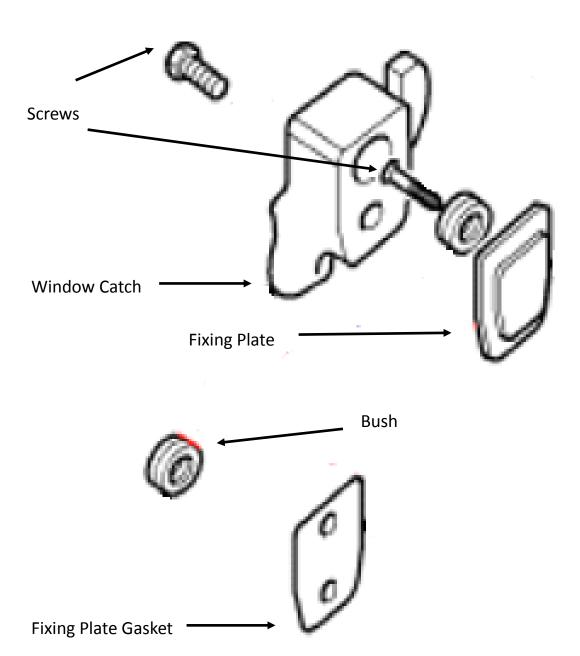
This diagram shows the assembly of a side window catch, and both the left and right hand sides fit together the same way. Please note that the bush will need to be gently hammered into place as it is a tight fit. The black painted screw is ideally used on the tapered end of the catch.
