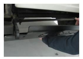
4. Adjust the distance between the left and right hand brackets to fit the holes on the back of the steering guard.
