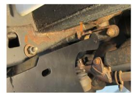
1. Remove the highlighted nuts from your vehicle in order to attach the left hand side bracket to the chassis.
