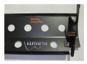
5. The brackets should fit to the rear of the steering guard as shown above.
