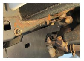
2. You may need to use a suitable penetrating oil to remove the nuts. If they are not present, use the nuts provided with the kit instead.
