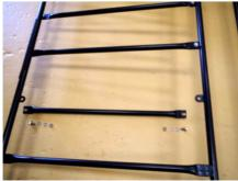
**6.** Using a nut, bolt and two washers for each bracket - as shown in the image - assemble the horizontal support beams on the front of the roof rack. If your vehicle has a sunroof then you can choose to leave these bars out.
