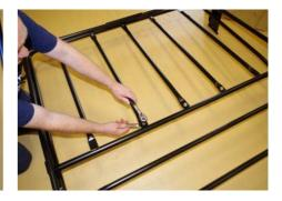
**7.** Ensure each bolt is fastened tightly, as this part of the roof rack will be taking most of the weight.
