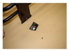
**5.** Insert the bolt as shown in the image above and apply the strip of protective rubber to the rear side of the bracket. This will be used to fit the legs to the guttering.
