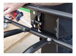
**2.** We recommend before you start to treat the welding joints with the black silicon sealant provided.
