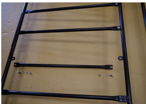
4. Using a nut, bolt and two washers for each bracket - as shown in the image - assemble the horizontal support beams on the front of the roof rack. If your vehicle has a sunroof then you can choose to leave these bars out.
