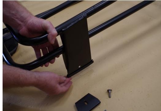
2. Fix the protective rubber strip to the base of each leg. This will protect the metal while it is on your vehicle and while you assemble the roof rack.
