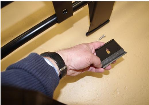
9. Using these brackets, fit each leg to the guttering of your Defender.
