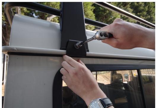
10. The brackets fit around the outside of the guttering and the legs slot inside the gutter itself. Ensure that the bolts are firmly tightened.
