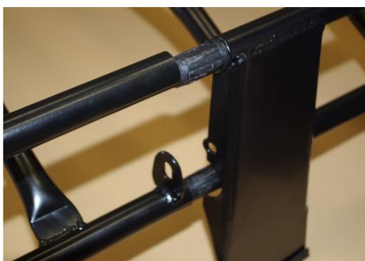
6. Connect the sections of framework together as shown using the ribbed rubber bungs provided. Before you insert the bungs, coat them in silicon (provided) to prevent any leakage. Use a rubber mallet to tap the pipes together as they are a tight fit.
