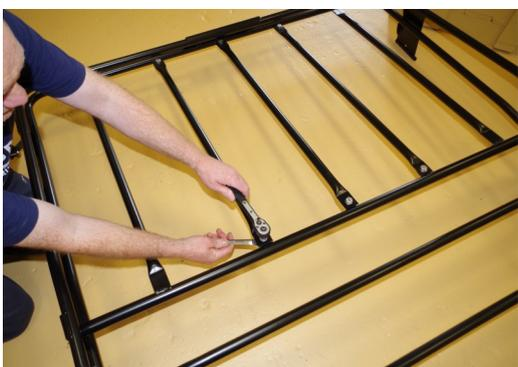
5. Ensure each bolt is fastened tightly, as this part of the roof rack will be taking the weight of a load.
