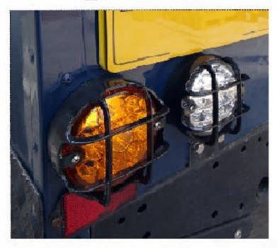
These guards will fit all of the 95mm diameter lights used on Defenders - fog, reverse and also NAS spec lights.
