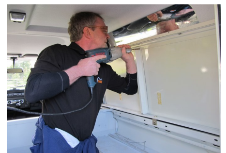
Drilling a pilot hole ready for cutting.
