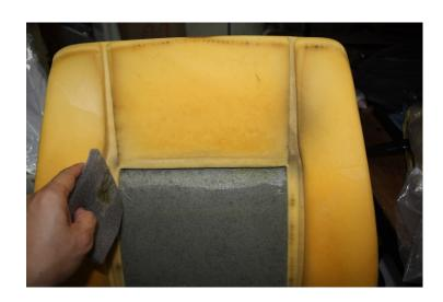
**7.** When the glue on both applied surfaces no longer feels sticky, carefully align them together as accurately as possible and attach. The adhesion should be firm by now.
