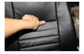
**11.** Use the C-hooks on the base unit to tie the seat covers underneath the seat frame where necessary.
