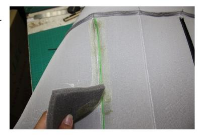
**6.** Apply the glue on to the upper seat foam in the areas which are to be attached to the seat cover.
