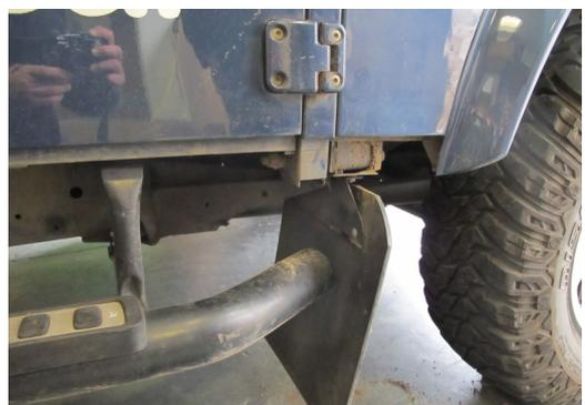
6. Check alignment of step; then tighten all nuts and bolts. The sills do not necessarily need to be removed.
