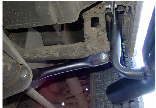
2. If your Defender has a fuel tank on the driver's side then the front fixing bolt should be pushed through from up behind the tank.
