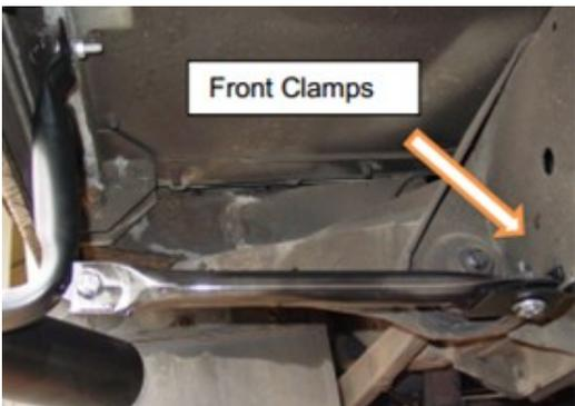
3. Fit the long front brace with clips underneath, and clamp to the edge of the tapered front chassis flange by the big rubber bush.
