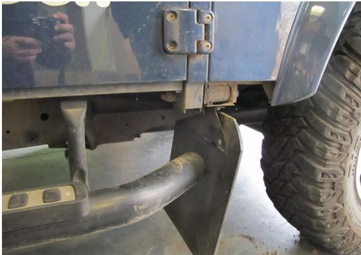
1. Offer the step into place on the outer edge of floor rails, the front hole is clear, the last rear hole in the rail needs the factory nut and bolt removing. The sills do not necessarily need to be removed.
