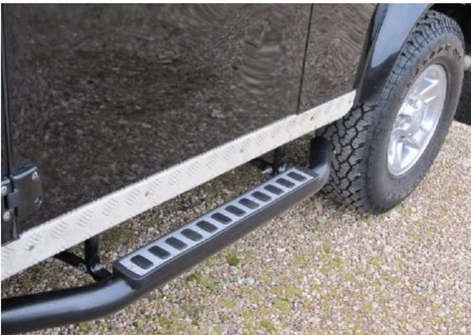
8. Test the step before you put it to use. Ensure all bolts are tight, and the tube lugs are correctly aligned. Although our steps are coated and galvanised to protect against rust, we recommend using Hammerite to coat the arms for additional longevity.
