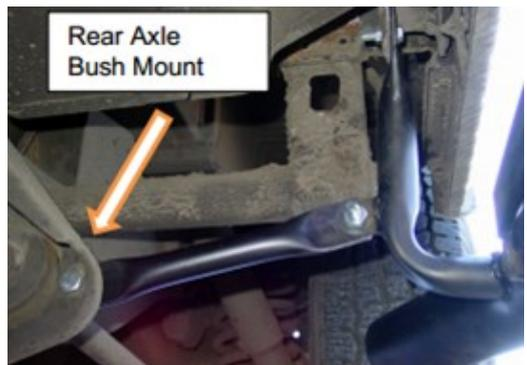
4. The short brace fits to the 17mm triangular axle support bush bolt, a new bolt is supplied if required.
