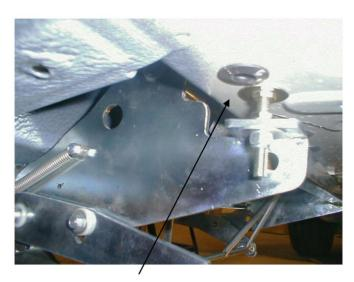
MAYBE NECESSARY TO DRILL Ø10 FIXING HOLE IN THE CHASSIS ALTHOUGH PREFERRED METHOD IS TO USE EXISTING CHASSIS HOLE
