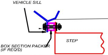
BOLT FRONT OF STEP TO VEHICLE SILL USING BOX SECTION PACKER (IF REQ'D) M8 BOLTS/NUTS &WASHERS
