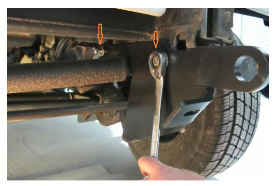
4. Adjust the right and left hand side bracket distance in between to meet the assembly holes on the main plate. Use the short bolts and nuts to fit the guard plate to the side brackets.
