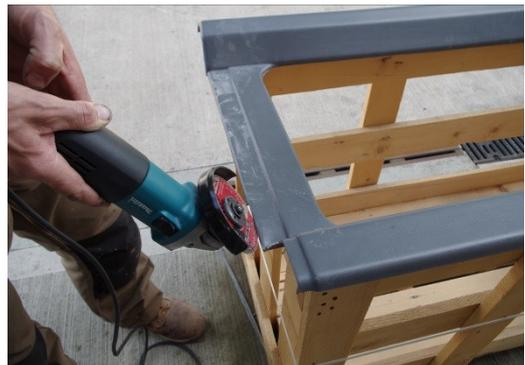
4. Offer all four trim panels to their respective surfaces. If the trim does not quite fit or is obstructed by anything on the interior of the vehicle, carefully file off any excess material with an angle grinder until the panel fits comfortably.
