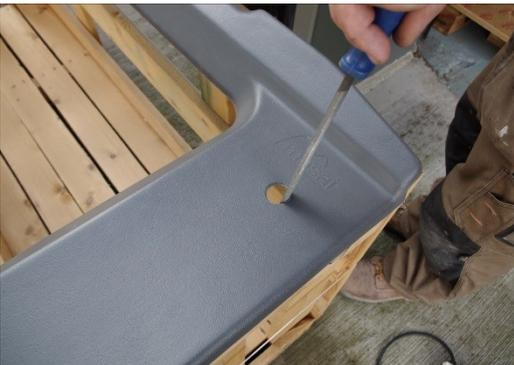
3. File the trim panels to remove any burrs or rough edges, taking care not to damage the material.
