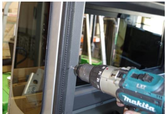
6. Set the first rear quarter panel in place and drill three small holes, as shown in the image above. Repeat this process on the other side of the vehicle.
