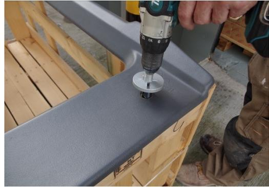
2. Offer each side trim up to your Defender and mark out the seat belt aperture points. Carefully drill out the points.
