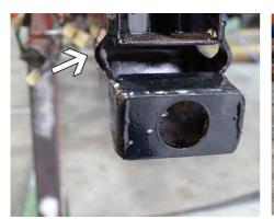
**STEP 4)** If you decide to cut these bulges, do the same on the left hand side of the chassis as shown above. **NOTE:** This bulge has no impact on the integrity/strength of your chassis.
