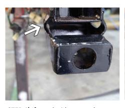
**STEP 4)** If you decide to cut these bulges, do the same on the left hand side of the chassis as shown above. **NOTE:** This bulge has no impact on the integrity/strength of your chassis.
