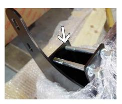
STEP 6) Our winch bumpers are supplied with heavy duty M12x120 high graded bolts. Standard Defender bumper bolts are M10 which can also be reused with our tubular bumper, however you will need to use a standard Defender nut insert on the underside to fit.
