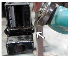
STEP 3) You may need to cut this outside bulge on your chassis with an angle grinder, they vary Defender to Defender and could stick out and interfere with the long arms of the tubular bumper. Cut only the OUTSIDE bulges. (RH side of chassis shown above). Once cut, touch up with black hammerite or red oxide paint to prevent future rust.
