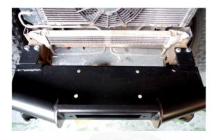
**STEP 7)** Once fitted, the tubular winch bumper should look like this on your chassis. **NOTE:** Photo shown is with the aircon extension brackets fitted.
