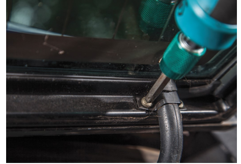
2. Unscrew the heated screen wiring covers, then disconnect connectors. The right-hand side may have wiring for the central locking actuator.
