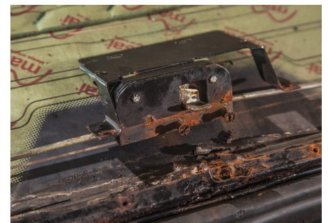
11. Unscrew the two screws holding the rod mechanism.
