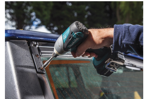
5. Undo the four tailgate screws, and remove the tailgate. We needed an impact driver to persuade my rusted bolts to move.
