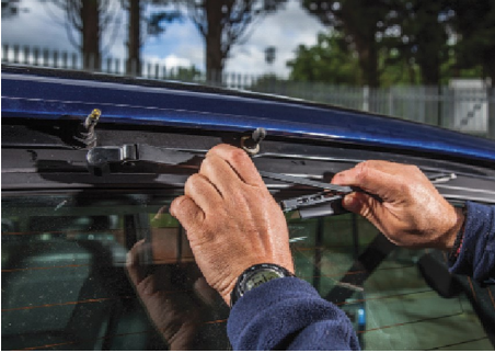
1. Remove the wiper arm, then soak the four tailgate hinges liberally in penetrating fluid.
