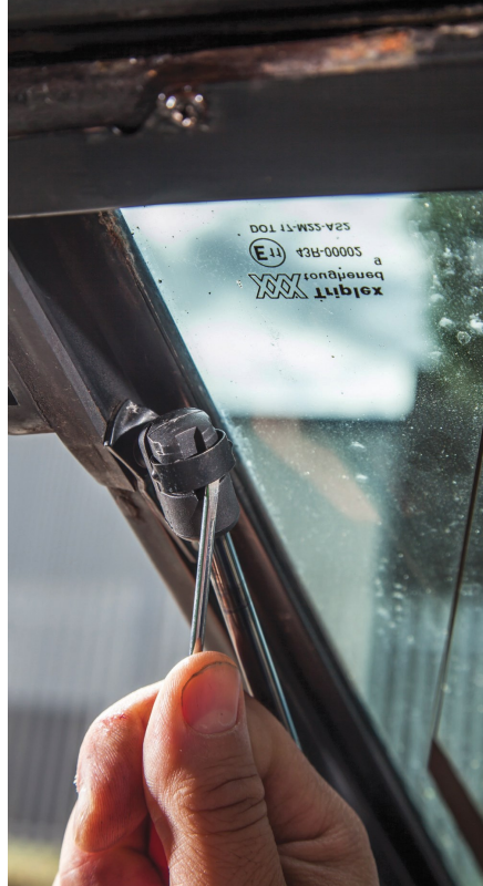
4. Release the tailgate struts, by putting a flat screwdriver under the clip. Remove the struts completely to avoid damaging the lower tailgate paintwork.
