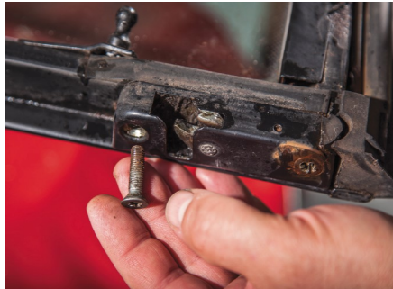
7. Due to rust, it can be difficult to remove the two catch screws.
