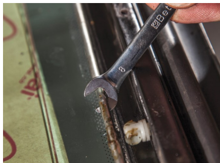
10. Prise out the lock rod clips, being careful not to damage the plastic. The actuators and mechanism are one part that can be very tricky to replace.
