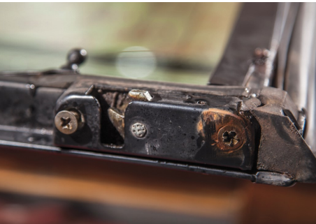
6. Working on the bench, the catches can be inspected. Ours were worn, but salvageable. You may wish to fit new replacements for peace of mind.
