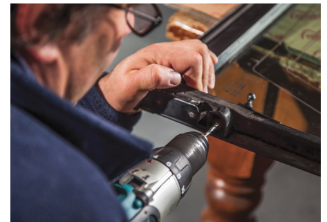
8. Be prepared to have to drill out most of them. A small pilot hole will make accurate drilling easier a second time with a larger drill bit.
