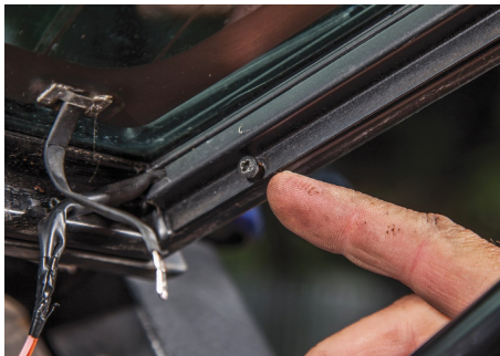
3. Remove screws on the metal cover down the right hand side and either side of the catches, and the plastic internal lock cover.
