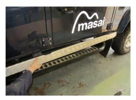
1) Remove your side sills. The side steps pictured are shown for illustration only and are not relevant to the fitting of tree sliders.
