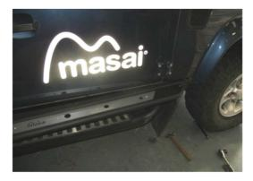
**5)** Attach the tree slider to the nut and align the front end. For Defender 90s, attach the slider to the bracket provided from step 4.
