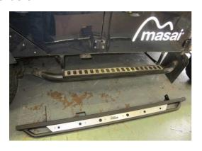
**3)** Align the tree slider along the side of the vehicle as above. Remove the bulkhead nut. You may need to push the bulkhead bolt out if you cannot get the slider into the correct position.
