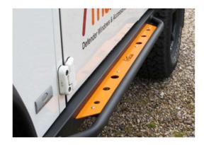
**6)** Push the back end of the tree slider into position, and bend the back bracket on the tree slider slightly to fit to the chassis and tighten bolts. For Defender 110s, you will need to drill two holes in the middle section on the outrigger to connect the tree slider.
