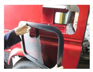
**3)** - Use a file to take off the sharp edges from the cut out surface and then offer the window to the vehicle to ensure that window is fitting correctly. (if you are fitting these windows to a vehicle with steel body panels, we recommend that you paint the edges with red oxide paint for rust protection).
