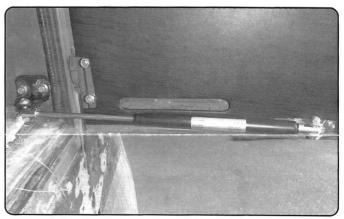
On post 2002 vehicles refit the door card and handle. On pre-2002 vehicles you will have to trim the door card before refitting it. On pre-2002 vehicles reposition the door card into place and mark out and trim the area wher the new bracket is fitted and cut out using a suitable tool. Position and refix the door card into place then the wiper motor cover and other covers and the door handle.
