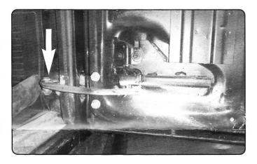
Undo pivot bolt and remove the door stay. Remove the pivot bracket on the inner wheel arch. Replace with the new bracket provided in the kit
