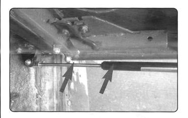
Fit strut loosely to the new pivot bracket. Position the strut against the door and open or close the door until you get a clearance at this point allowing for clearance of the door card to fit on pre-2002 vehicles and so that the strut does not get damaged during operation on all ages of vehicles.
