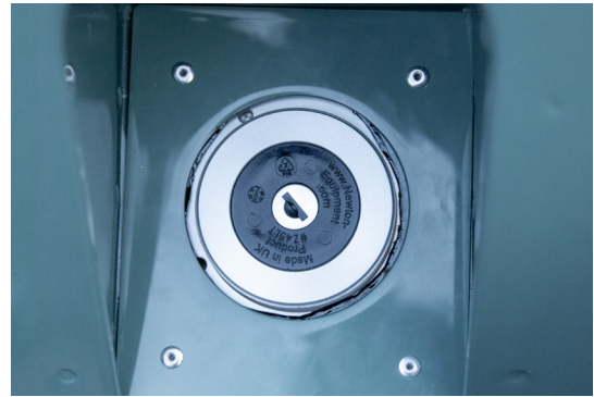
14. Push the internal section of the fuel cap through from behind with the aluminium threaded ring attached.
