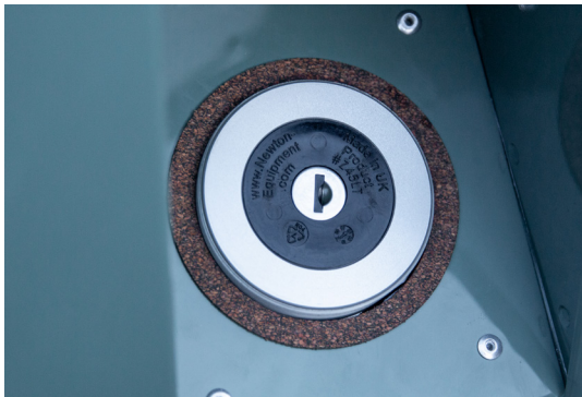
15. Holding the internal section of the cap in place lay the cork gasket over the cap.
