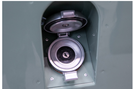
16. Screw the top of the cap down onto the internal section until tight and the top of the cap lines up like the picture.
