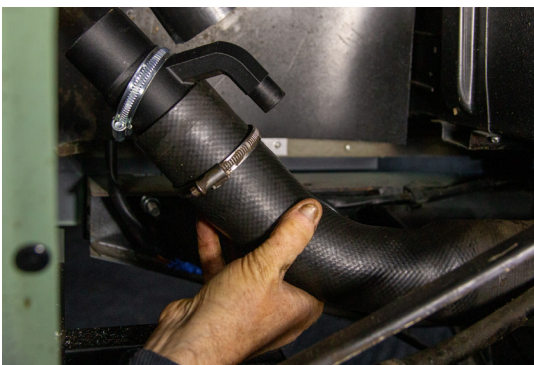
17. Connect the filler, breather tubes and the hard pipes together.
