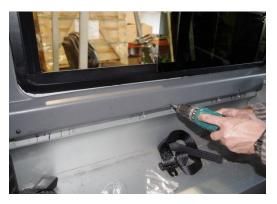
8. Using three long screws in the locations shown in the image above, fix each side panel in place. Take care not to over tighten these screws as the plastic could crack.
