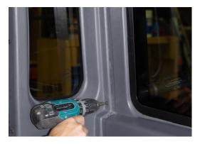
11. Fix the rear quarter panels to the side panels using two short screws on each side. Be mindful that you do not exert excessive pressure on the plastic.
