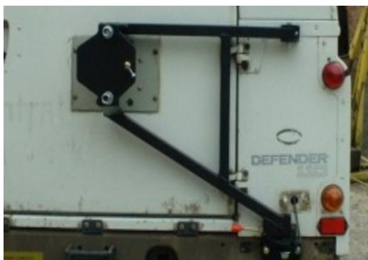
3. With the top tube level, mark the position of the two holes on the bottom bracket and the right hand bracket of the top bracket.
