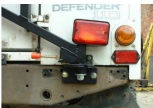
5. Remove any trim or wiring from behind these marked positions and then centre punch and drill through using a small drill bit.
