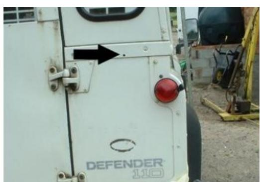
6. Enlarge the top holes using a 7mm drill bit to accept the 6mm bolts and use a 10.5mm drill on the cross member to accept the 10mm bolts, making sure you drill through both sides of cross member.
