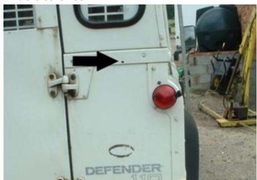
4. Remove the wheel carrier and measure the distance between centres of top bracket holes. It should be 40mm. Use this measurement to mark the position of the other hole in top bracket.
