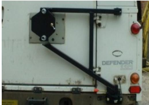
1. Place the wheel carrier in position with the bottom bracket on the rear cross member straddling the body lug.
