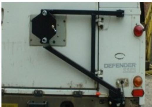
9. Open the wheel carrier and place the two M6 bolts Hex bolts through the holes in the top bracket and fit the backing plate on the inside between the body and the nuts.
