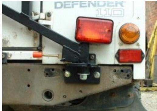
7. Remove any burrs and touch up any bare metal with paint.
