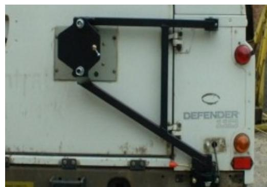
10. If required, two additional holes can be drilled through the backing plate using a 7mm drill and the bracket can be secured using the two M6 Posi-head bolts.
