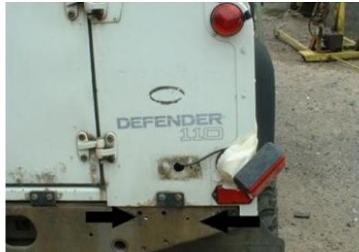
2. Make sure the top bracket is level and over the reinforced joint between the body tub and the hardtop or canvas tilt. Note, if the vehicle is fitted with a rectangular rear fog light, this may need to be raised to provide clearance.
