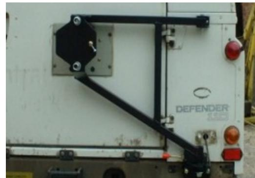
8. Place the wheel carrier in position and using the two M10 bolts, bolt the bottom bracket to the cross member using the backing plate between the cross member and the nuts.
