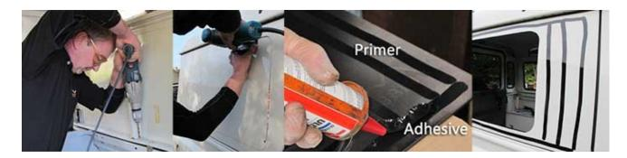
Once you are confident you can cut out the aperture accurately, drill a hole for the blade near the marked line, within the marked area in the chosen place you want to start cutting.
