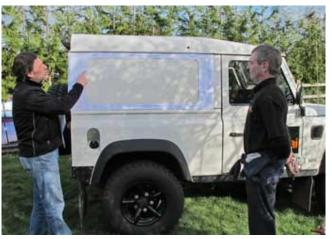
accurately draw the section to be cut out following the inside edge of the template.
