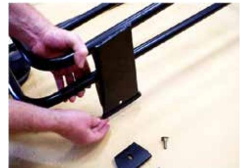
**4.** Fix the protective rubber strip to the base of each leg. This will protect the metal while it is on your vehicle and while you assemble the roof rack.
