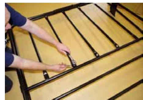
**5.** Insert the bolt as shown in the image above this will be used to fit the legs to the guttering.
