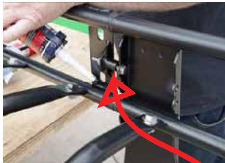
**2.** We recommend before you start to treat the welding joints with a black silicon based sealant. (not included)
