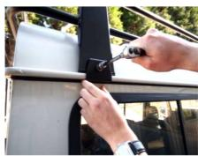
**12.** The brackets fit around the outside of the guttering and the legs slot inside the gutter itself. Ensure that the bolts are firmly tightened.
