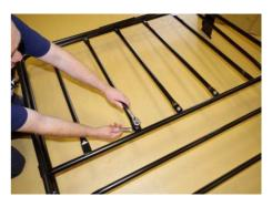
**7.** Ensure each bolt is fastened tightly, as this part of the roof rack will be taking most of the weight.
