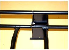
**9.** Fasten a bolt through the bracket to hold the sections together.
