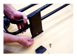
**4.** Fix the protective rubber strip to the base of each leg. This will protect the metal while it is on your vehicle and while you assemble the roof rack.
