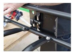
**2.** We recommend before you start to treat the welding joints with a black silicon based sealant.
